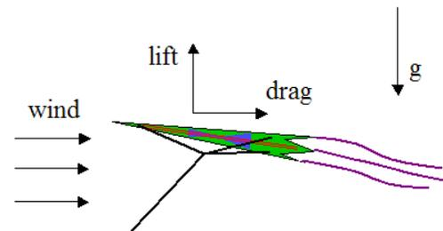
The lifting force is (relatively) weak, which is why kites need to be made of lightweight materials. Kites sometimes need a bit of supplemental force in order to take flight, this means creating **apparent wind**, by running and pulling the kite behind you.
