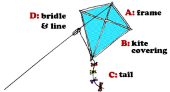
Kites are not like rockets, propelled into the air by a physical or chemical force from below, and they aren't like a paper airplane or parachute, coasting on air-resistance. Kites actually work remarkably like an airplane when they are in flight. Instead of using powerful engines to create **lift**, the kite relies on the force of wind blowing towards and underneath the kite to create **lift**.
