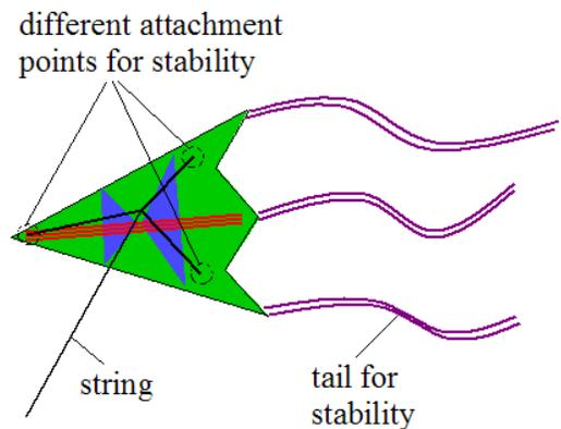
Wind moves across the surface of a kite and creates pressure. **Lift** results from the pressure being deflected along the face of the kite. In other words, the wind pushes up on the kite. Think of wind pressure like a hand, pushing the kite up into the sky and holding it there.
